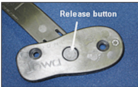
Figure 3. Iowa Brace platform
